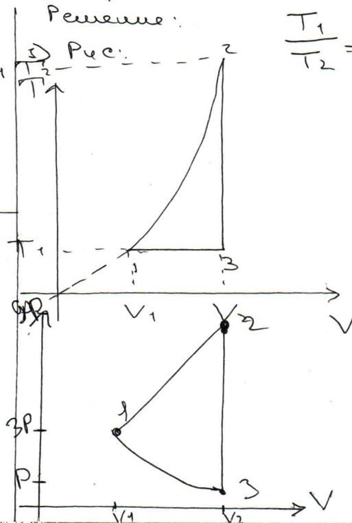
$$\frac{T_1}{T_2} = \frac{kV_2^2}{kV_1^2} = \frac{1}{9} \Rightarrow T_2 = 9T_1.$$
