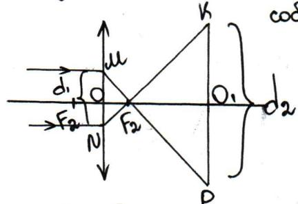
$$\Delta M F_2 O \sim \Delta K F_2 O, \text{ но } 2L \\ \frac{d_1 \cdot d_2}{2 \cdot d_2} = \frac{O F_2}{O O_1 - O F_2}$$
